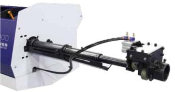
The first roller steady rest is mounted internal to the front of the bar feeder providing support to the bar as it enters the telescopic nose.
