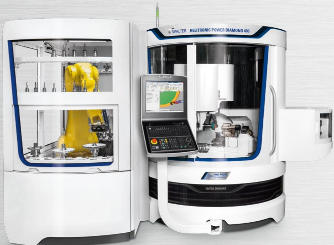
HELITRONIC POWER DIAMOND 400 with the "Robot loader 25" (left) and "Electrode/grinding wheel changer" (right) options – the ultimate configuration for high performance
