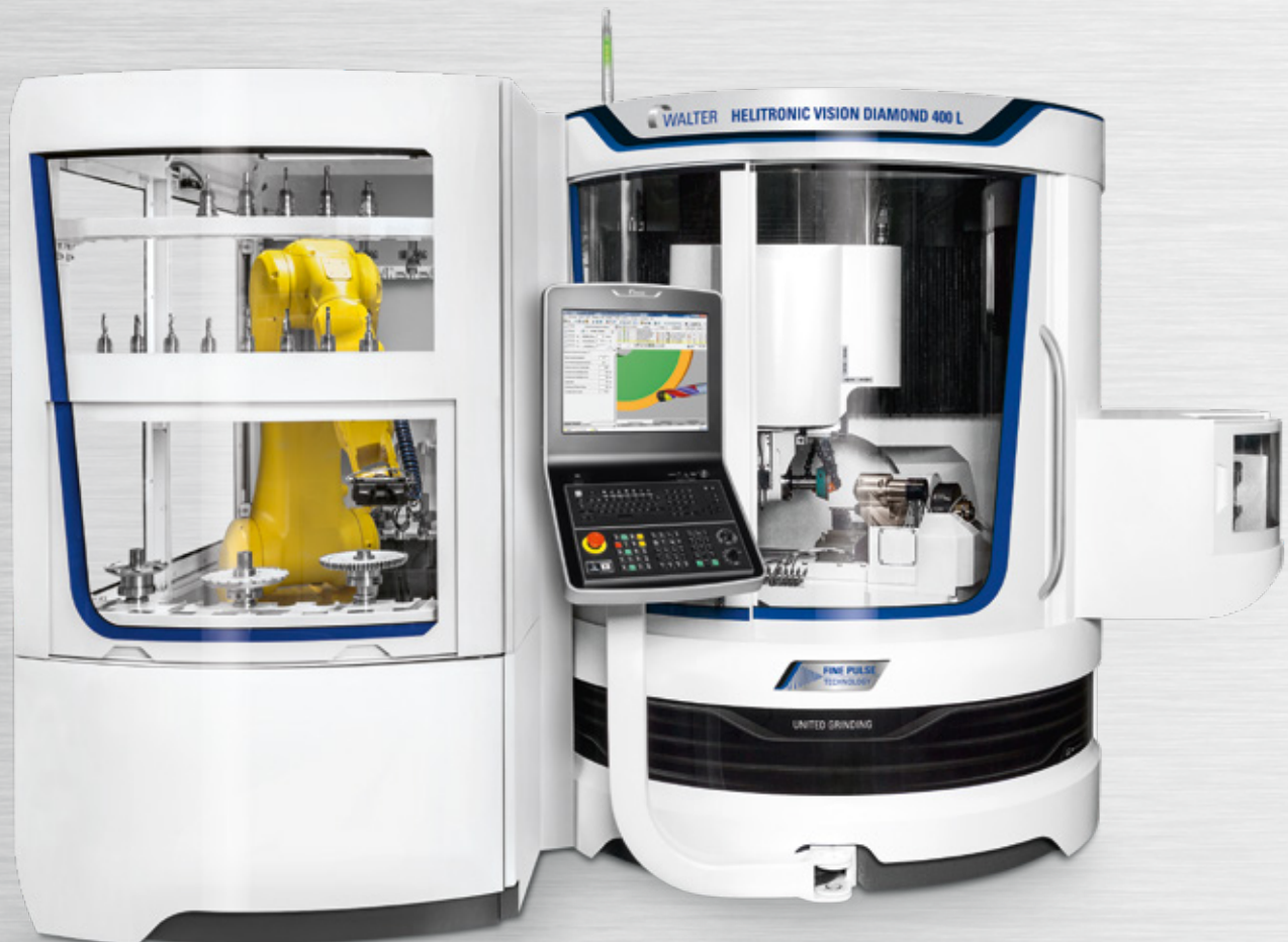
HELITRONIC VISION DIAMOND 400 L with the "Robot loader 25" (left) and "Electrode/grinding wheel changer" (right) options – the ultimate configuration for high performance
