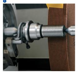
The optional C-axis enables thread and form grinding, increasing the machine's potential applications. A controlled power chucking cylinder which actuates power chuck and spring collets is available for automatic workpiece clamping.
