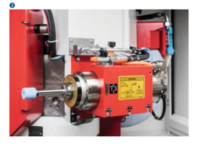
The swiveling wheelhead is equipped with water-cooled, roller-based, and maintenance-free motor spindles with stepless speed control and the latest generation of contact sensors. The shaft ends hold external wheelheads with a diameter of 500 mm (20") and a width of 63 (80 F5) mm (2.48" (3.15" F5)). For internal grinding, use powerful high-frequency spindles with 120 mm (4.72") external diameter. It's your choice: configure the wheelhead to match your specific needs.
