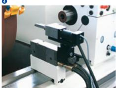
The length positioning measuring head is suitable for the passive length positioning of interupted or non-interupted surfaces. It has an electric or pneumatic probe lift-off and uses one measuring circuit.
