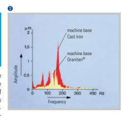
Granitan® S200 slideway coating. The patented knobbed structure of the guideways largely eliminates the slip-stick effect or floating of the slides observed on conventional guideways. The guideways offer the highest possible accuracy through the entire speed range with high load capacity and dampening levels. Thanks to the robust and maintenance-free design, these excellent guideway characteristics are more or less completely retained.
