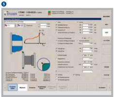
Two different operating systems are available, StuderSIM and StuderWIN. Both operating systems are suitable for a wide variety of internal grinding applications and enable reliable programming of all basic cycles for grinding, dressing and processs-supporting measurement. The basic cycles such as face grinding, bore grinding, taper grinding, thread grinding, dressing and gauging are defined in the Parameter Input window. This type of programming
