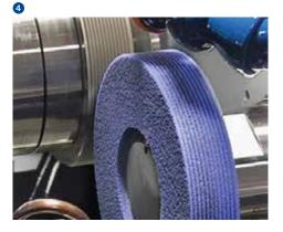
The wide variety of dressing options enables optimal adaptation of the machine to the most diverse applications and workpiece requirements. In addition to fixed dressing units, devices for rotating dressing tools can also be mounted. The latter are especially suitable for dressing ceramic-bonded
