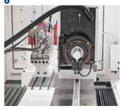
Cones and tapers can be machined in two ways. Either by using a swivelling work table with a manually adjustable range of up to 21 deg (31 deg for S110) or with a fixed table and an appropriately dressed conical grinding wheel.
