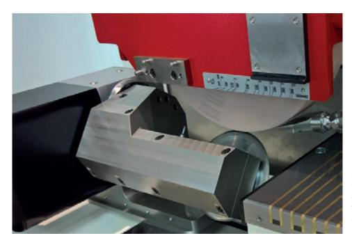
**Swivel dresser** PA-T130 mounted on the left of the machine table. Torsion-resistant dressing arm mounted on one side for a  $\mu$ m-accurate contour and fast tool change. Automatic adjustment of the dressing wheels (profile depth up to 30 mm).
