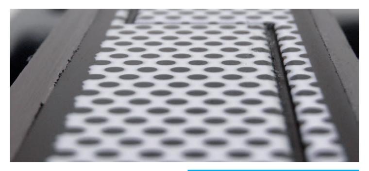
Optimal dampening and maximum smoothness increase the precision of the grinding process. To achieve this, the J600 is equipped with scraped guideways in the X-axis and the guides on the table base with the new EasySlide coating. As a result your parts receive a very high surface finish quality. The new wear resistant composite EasySlide coating on the lateral guides and on the table base ensures utmost running smoothness, increased precision and high surface finish quality.
