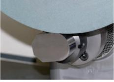
and noncircular grinding tasks can also be performed with the highest precision and surface quality.
