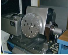
Double CNC indexing table for 5-axis continuous path controlled profile grinding
