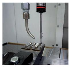
**Measuring probe,** pneumatically retracting from measuring position, measuring accuracy ±1 µm
