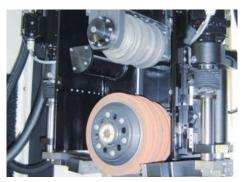
Overhead dressing system PEA-K for IPD and CD grinding methods designed for a grinding wheel width of up to 200 mm.
