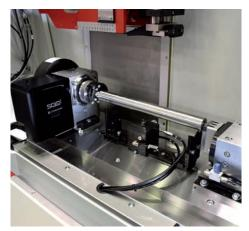
**NC indexing table,** 1 or 2 axis, indexing accuracies up to ±1"
