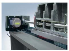
**Z-axis,** with linear glass scale
