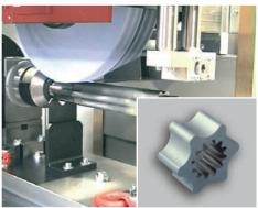
Outer-profile of hydraulic pump rotor
