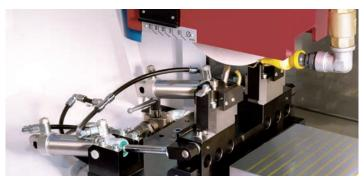
**Tilting dressing attachment** for circumferential, face and profile dressing. The attachment is pneumatically actuated and is tilting down to avoid collision with the grinding wheel and wheel guard during the grinding cycle.
