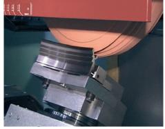
Shroud segment — multiple operations in 1 set-up
