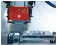
**NC-tilting magnetic chuck,** tilting range +/-30° indexing accuracy +/- 1"
