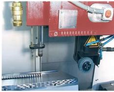
Measuring probe, pneumatically retracting from measuring position, up to 2  $\frac{1}{2}$  axes, measuring accuracy +/- 1  $\mu$ m
