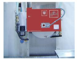
**Vertical auxiliary grinding spindle** for universal use in the mould and die industry with a power of up to 6 kW and up to 90,000 rpm
