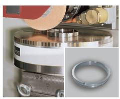
Grinding of anti-rotation slots
