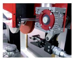
New way of grinding wheel cleaning, with newly developed nozzle positioner, 30% less grinding wheel wear, 30-40 bar nozzle pressure
