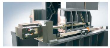
**Z-axis,** direct drive with linear glass scale
