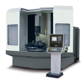
$\label{lem:profile} PROFIMATMC610VS\,with\,vertical\,grinding\\ spindle$
