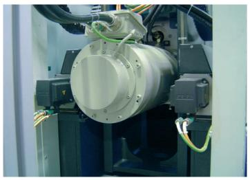
Z-axis with parallel drive system for increased rigidity (optional)
