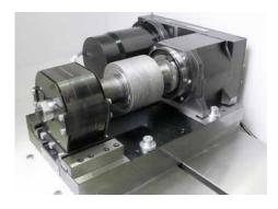
Table mounted dresser type PA-TL 200S for diamond rolls up to a width of 200 mm or for contour dressing with universal diamond dressing disks and a rough dressing disk.
