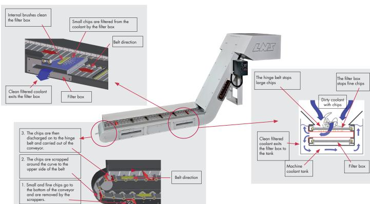
Large, stringy chips are stopped and taken out by the continuous hinge belt conveyor.
