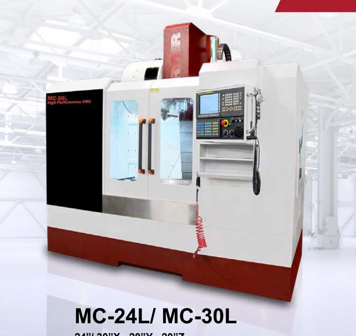
24"/ 30"X 20"Y 20"Z 20" x 28"/ 35" Table Size 1,450 IPM Rapids 30 HP - 40 Taper Inline Spindle 60 - 10,000 RPM 30 Station Arm Style ATC
