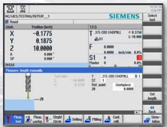
Touch off the tool on the part or use the available quill scale to get a real feel of the tool on the part. This process can also be done automatically with available tool probes.
