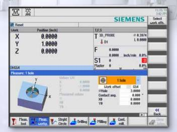
Several standard cycles are available to find centers of holes, part edges, and bosses. Cycles can also be used to measure finished parts and display the reading.
