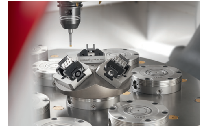
Inserting grooves with the TENDO E compact
